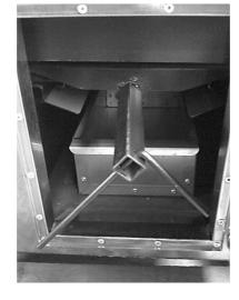
firing regime adjusting mechanism with regime adjustment spanner (24)
