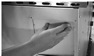
Remove the sheet beneath the lid by pressing onto the weakest juncture
