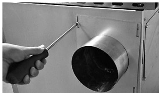
Install the external protective sheet by using bolts previously used to attach the external protective lid
