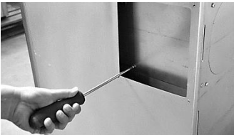
Remove the internal protective lid with a screwdriver
