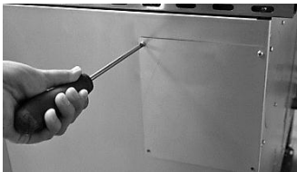
Remove the external protective lid with a screwdriver
