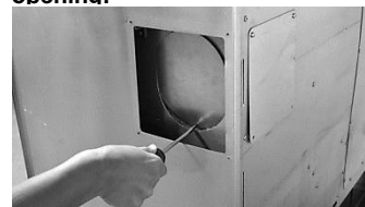
Remove the sheet beneath the inner lid by pressing onto the weakest juncture
